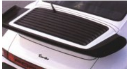
Turbo 3.3 output 300 hp. Higher rear wing housed the intercooler.
