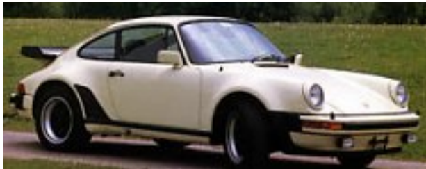
Turbo 3.3 output 300 hp. Higher rear wing housed the intercooler.
