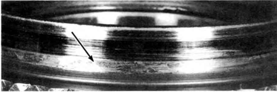
Metal transfer from synchronizing ring
