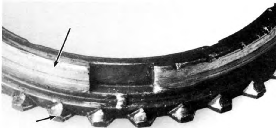
Worn synchronizing ring and damaged teeth
